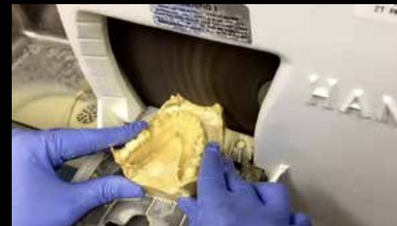
11. Trim/grind off excess material
